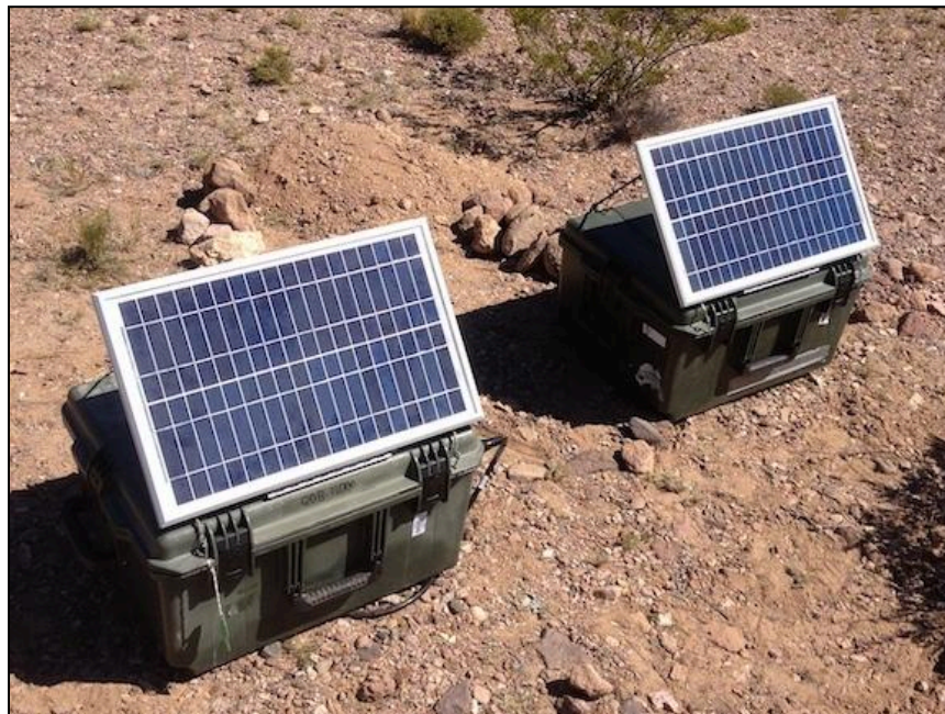
Figure 2: The Pelican iM2750 Storm Travel Case modified for a temporary seismic deployment.
