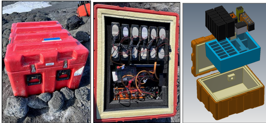
Figure 9: The SAGE semi-permanent power system enclosure used in Polar applications.
