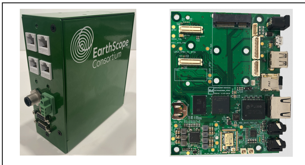
Figure 14: The Nitrogen8M_Mini, a 4 port switch and a power supply in a custom EarthScope enclosure.
