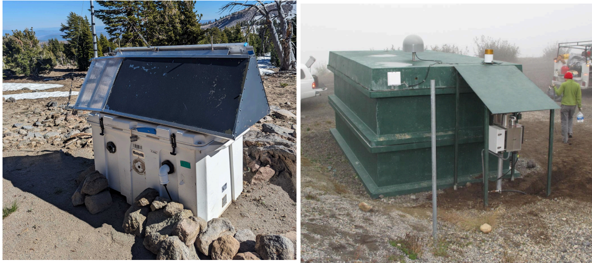
Figure 12: These types of ruggedized enclosures prevent buckling in heavy snow accumulation zones.
