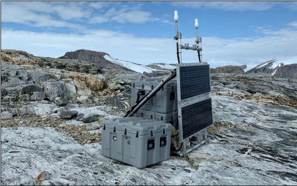
Figure 4: The Hardigg enclosures used in polar environments can hold up to ten large batteries. These cases weigh down the aluminum structure.
