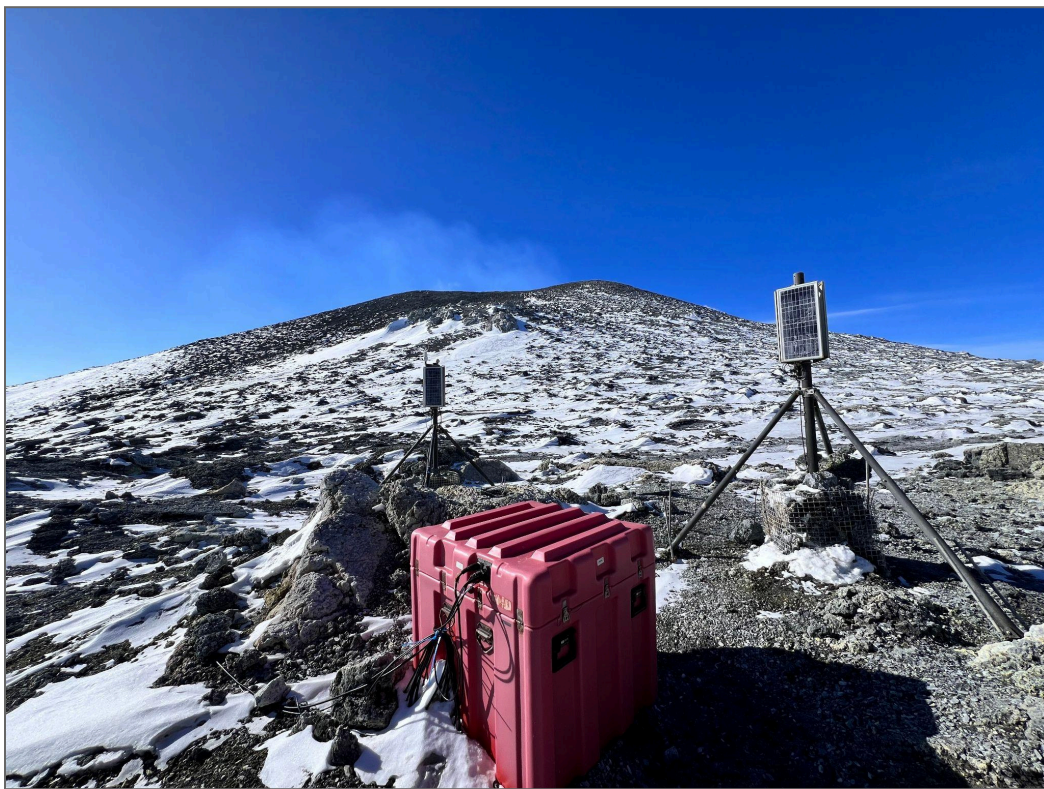
Figure 5: A SAGE semi-permanent enclosure. This enclosure is insulated with double-layered vacuum insulated panels with a sealed acrylic lining encasing them for protection.
