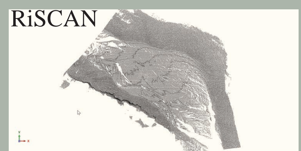
Figure 10: Visualization of a LiDAR point cloud in RiSCAN showing outline of Garwood Valley in Antarctica.
