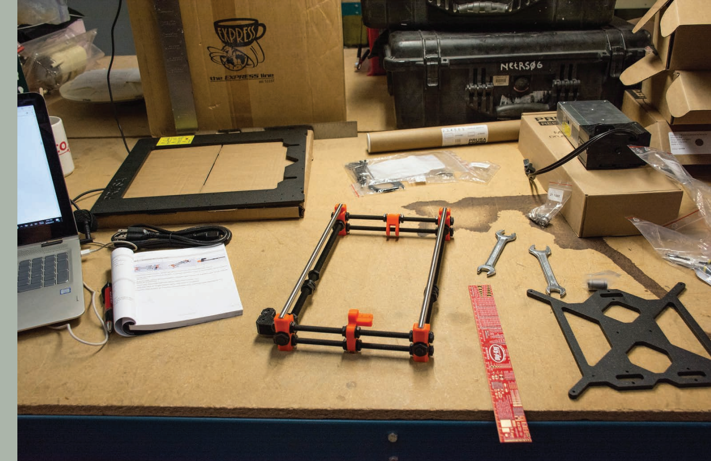
Figure 2: The Prusa i3 MK2 during assembly showing completed y-axis.
