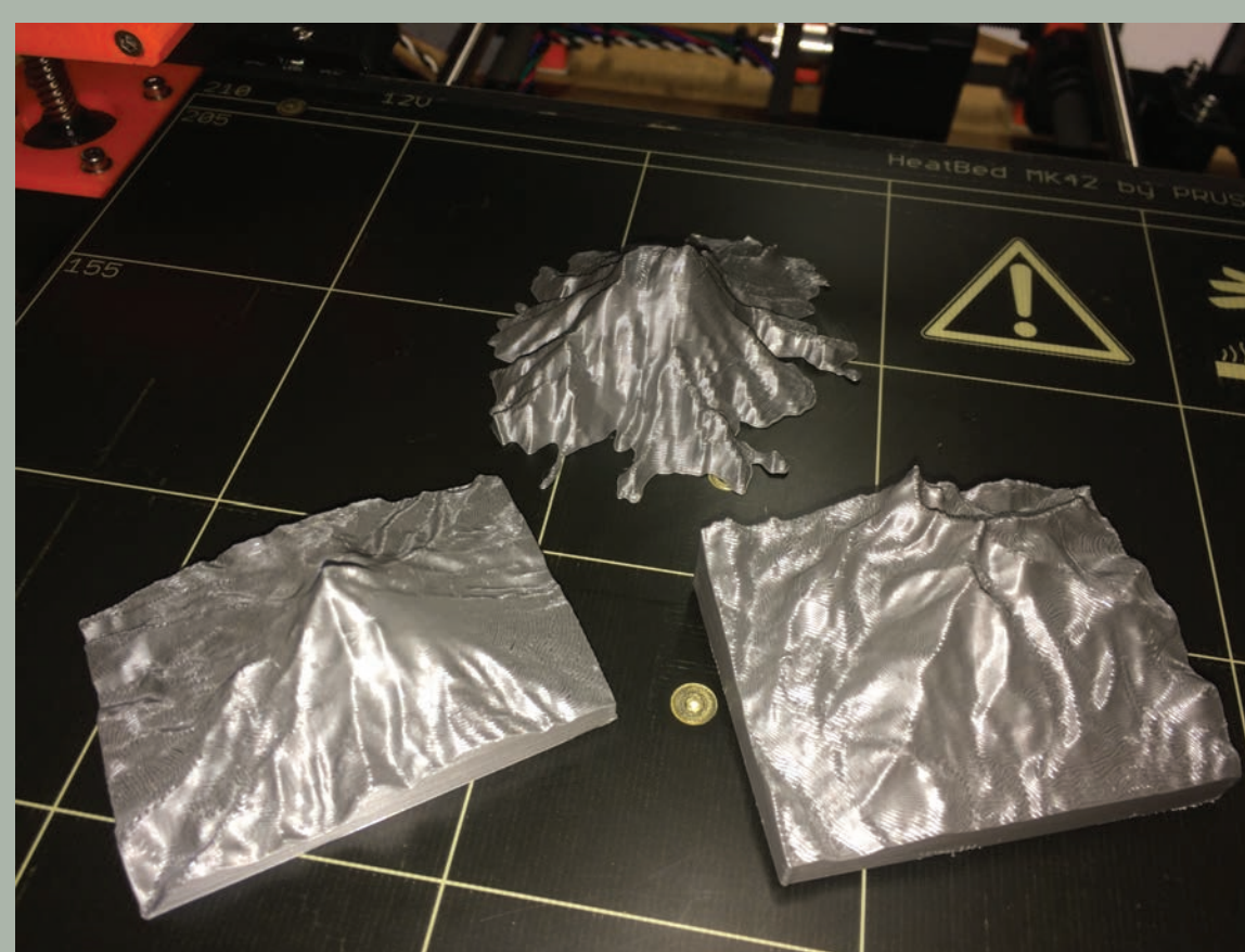
Figure 15: Mt Hood created from Terrain2STL. Mt Pelée created from Thingiverse, Longs Peak created from OpenTopography.
