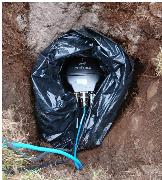
Figure 1: Certimus digital seismometer being deployed as an angle in a shallow direct burial installation.
