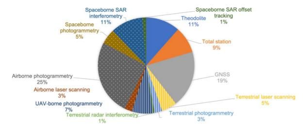
Percentages of the different techniques adopted for measuring or computing rock glacier velocities in the literature. The solid, striped, and dotted areas represent in-situ, close-range remote sensing, and remote sensing techniques, respectively.
