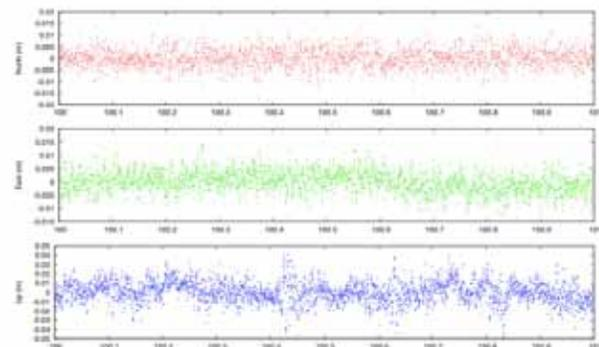
**Figure 2.** Kinematic processed baseline positions between P804 (deep drilled monument) and P805 (short drilled monument) for one 24-hour period (2013 Day 100) using the TRACK software. The baseline residuals for three components North, East, and Up are displayed in meters.
